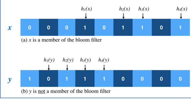
Fig. 5. Example of Bloom filtering elements  $x$  and  $y$
