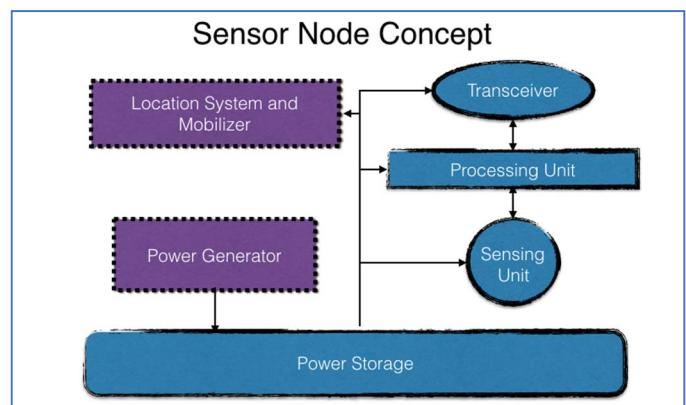
Fig. 1. Simplified components of a sensor node
