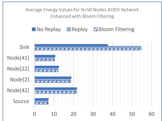
Fig. 7. Energy levels in different nodes in no-replay, in replay, and with Bloom filtering
